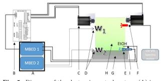
Fig. 5 Diagram of the electronic control system. (A) is an electronic box with 2 MBED microcontrollers. The first one controls the variators (B) of the motors (C) and the photoconductive cells (E), the second one controls the humidity captors (D), placed respectively at the top and at the bottom of the film. (F) is the spectrometer, (G) is the tank, (H) represents a soap film. This scheme is not to scale
