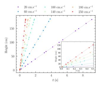
Fig. 6 Altitude reached by the fishing line as a function of time. The dots represent measurements made with a high-speed camera with a frame rate equal to 125 for velocities between 20 and 140 cm s<sup>-1</sup>, and a frame rate equal to 250 for the velocities 180 and 250 cm s<sup>-1</sup>. The dotted lines correspond to the theoretical height  $V \times t$ . The inset is a zoom of this graph at short times, for t < 0.5 s
