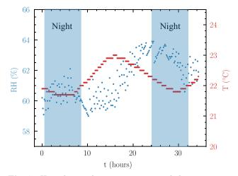
Fig. 7 Humidity and temperature recorded over time in the enclosed box for 30 h, for an experiment performed at  $\rm RH=60\pm4\%$
