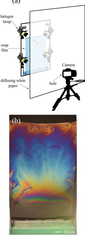
Fig. 10 a Experimental setup used to visualize soap films. **b** Photograph obtained by using this set-up with a Nikon D7200 camera and a large angle objective lens. The film is generated at a velocity of 50 cm  $s^{-1}$  at a height of 120 cm with a 4% Fairy solution
