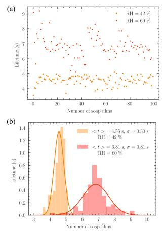
**Fig. 8** a Lifetime measurement of 100 soap films along an experiment performed at a velocity of 20 cm s<sup>-1</sup> with controlled humidities of 42% and 60%. The soap films break during their generation. **b** Histograms obtained for these two experiments. The lines represent the normal distribution
