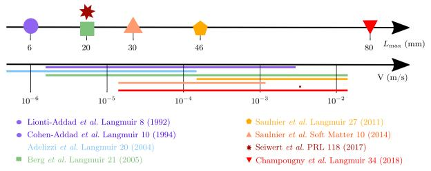
Fig. 1 Schematic diagram of the range of maximum lengths and velocities studied in the literature for soap films generated by pulling a frame out of a liquid bath
